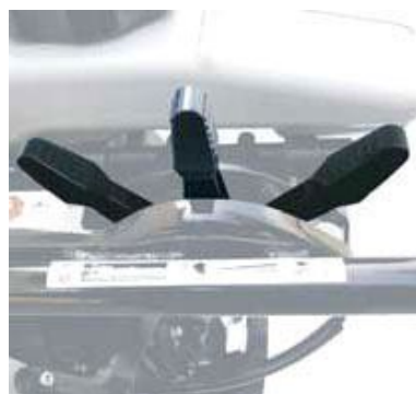
Throttle lever with a kill switch interlocking with fuel cutoff mechanism.
